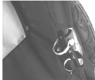
Swing the crossbar upward into position across the top between the side panels and route it through the loops at the top of seat. Insert the crossbar into the upper sleeve and lock with the safety pin.
