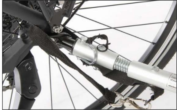
To disconnect the trailer, loosen the safety pin and the safety strap. To dismount the connecting bolt, unscrew the rear hub nut.
