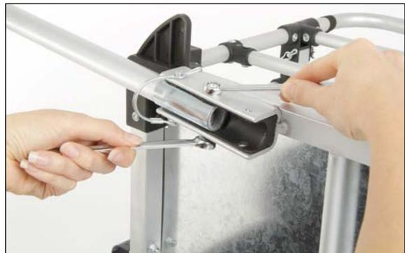
To stow the trailer drawbar, reverse the steps and secure the safety pin with the clamping spring.
