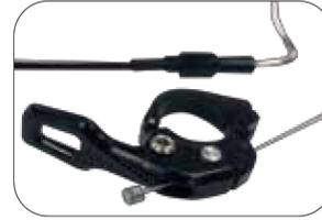
4. Insert the cable into the cable housing.
