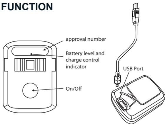
1. When the green battery level indicator light turns on, the rechargeable battery must be charged immediately. While charging, the level indicator shows a red light which turns off when the rechargeable battery is fully charged. Charging time about 2-3 hours
