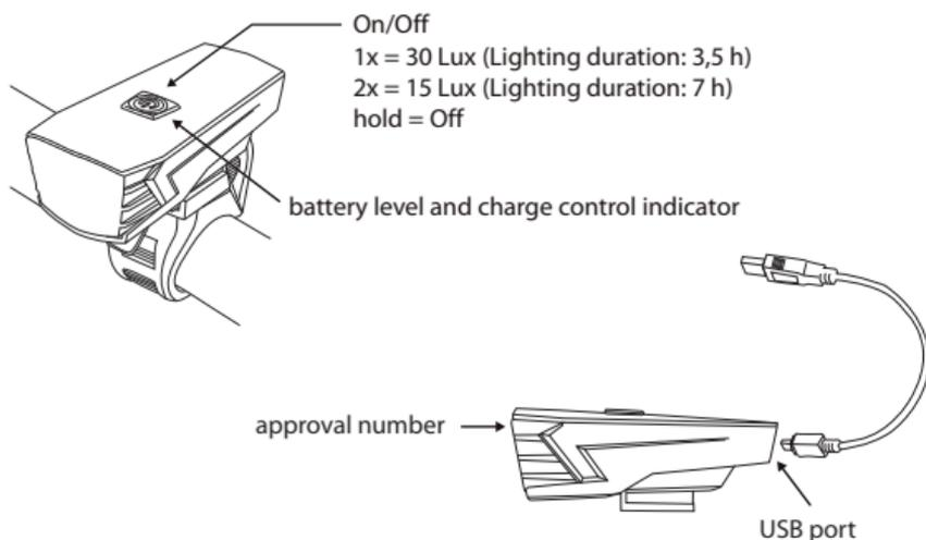
1. When the red battery level indicator light turns on, the accumulator must be charged immediately. While charging, the level indicator shows a green light which turns off when the accumulator is fully charged. Charging time: approx. 3 - 4 hours
