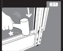
To prevent the anchor from becoming loose, ensure that the two angled attachment tabs above the hooks firmly hold the pillar in place. Note: Use a hammer to tap the anchor into place for firm assembly.
