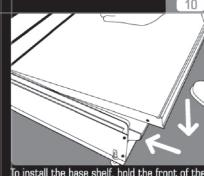
To install the base shelf, hold the front of the base shelf with both hands, lift the shelf up at a 45° angle and insert the plate at the back of the base shelf into the groove in the lower anchor until it clicks into place. Place the back panel in a horizontal position and make sure the tenons at the back of the shelf are securely featered into the School halos in the page fastened into the S-shaped holes in the anchor.
