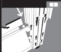
Put the pillars in place; use one hand to insert the hooks on the back of the lower anchor into the holes near the bottom of the pillar and oush down to lock.
