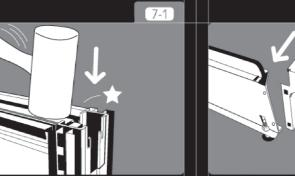
To install the base front, put the holes on one end of the base front over the hooks on one foot stand plate and push down to lock into place; install the other end the same way.
