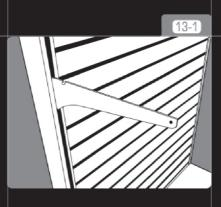
Put the shelves in place. Hold up the front edge of the shelves in place. Hold up the Holt edge of the shelves roughly at a 45° angle and position the side plates on both sides of the shelves over the outsides of the brackets; lower the shelves into position and make sure the tenons are in place.
