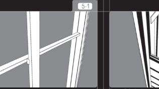
To install the back panel (either slat wall or pegboard) push the two sides of the pre-installed back panel into the grooves in the pillars in an upwards direction and then push down to lock into place.
