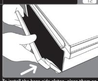
To install the base side plates, place them on the foot stand plates, and insert the hooks at the front of the side plates into the holes used to attach the base front. Insert the lips on the pillar side covers into the grooves in the anchors and push down to lock into place.
