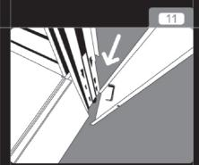
To install the pillar side covers, insert the hooks inside the side covers into the holes in the pillars and push down to lock into place.
