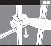
To install the slat wall's central back pillar, insert the bottom of the pillar into the slot in the foot stand plates.
