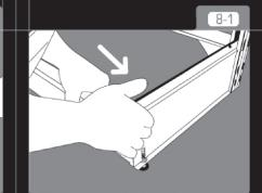
Make sure that the hooks on the top of the base front are firmly inserted into the holes on top of the foot stand plates when installing the other end of the base front.
