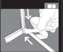
Insert the hooks at one end of the foot stand plate tightly into the holes on the side of the pillar and push down to lock into place.
