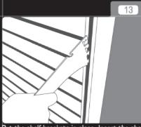
Put the shelf brackets in place. Insert the shelf brackets into the desired holes and push down to lock the hooks into place.
