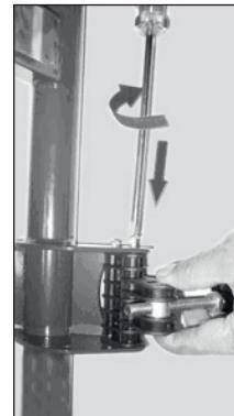
3. To fasten the magnetic wheels with the given tools.
