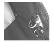
Swing the crossbar upward into position across the top between the side panels and route it through the loops at the top of seat. Insert the crossbar into the upper sleeve and lock with the safety pin.
