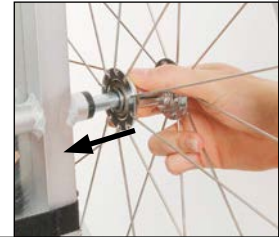
b) insert the axle in the opening
