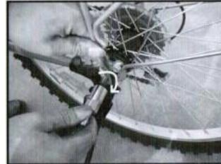
For bikes that don't use the quick release, tighten the screw.
