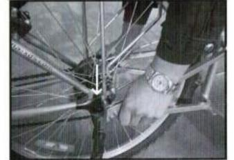
Attach the assembled trailer to the quick release mechanism.
