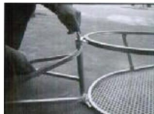
Secure the trailer frame to the front fork using the connecting spindle.
