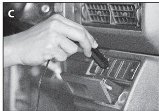
2) Plug the power cord into the cigarette lighter receptacle (Fig. C) or connect it to the power adapter to use a different power source. Then set compressor on/off switch to "on" position.
