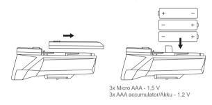
Attention! Insert correctly (+/-). Do not charge, do not disassamble, do not dispose of in fire, do not short circuit. Keep away from children. Do not use following batteries at the same time: old and new, half full and full, different brands and capacities. Remove immediately from device if not in use or the batteries are empty. Dispose of defective and empty batteries properly (hazardous waste).
